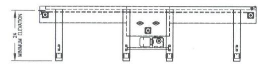
NARROW WAY = 36", 48", 60" & 72" CHAIN WIDTHS WIDE WAY = 84", 96" & 120" CHAIN WIDTHS
