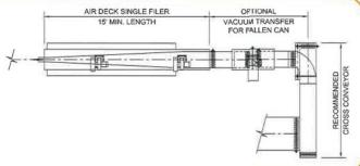
"Stripper" continuous motion indexing discharge for non-round containers (other than glass). An efficient and cost effective method to single file non-round containers that have been palletized in rows (brick pack). This style of single filer is usually integrated to the sweep of the
